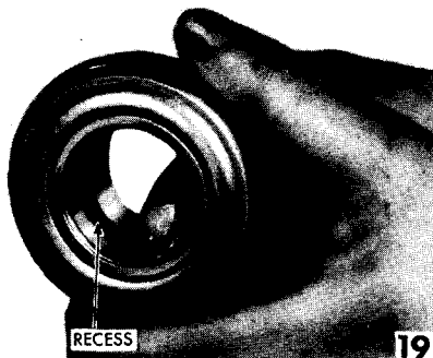
CLUTCH RELEASE BEARING SUPPORT—WB Fill recess inside of release bearing support with grease. Lubricant should be level with edges of recess.
